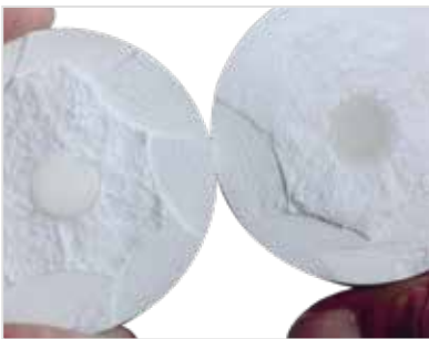
d) Separated investment ring at transition point from plunger to pressing cone.
