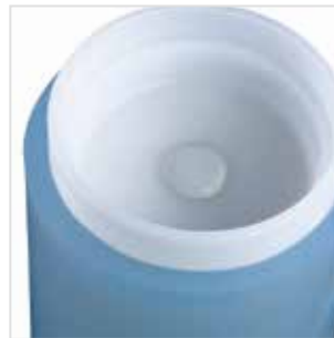
c) Once the investment material has set, remove the ring.
