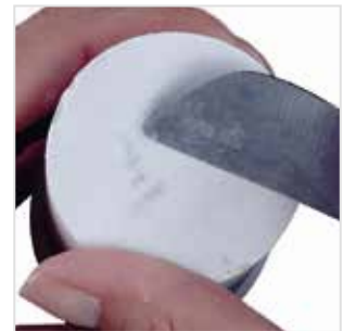
d) Using a plaster knife, smooth out any unevenness.
