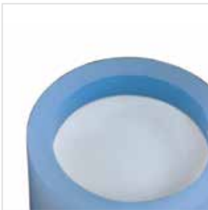
a) Pour investment material into the ring with slight vibration.
