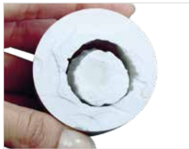
e) Rough divesting with \text{Al}_2\text{O}_3 at max. 4 bar pressure. Careful, precise blasting with glass beads (medium grain size) at max. 2 bar pressure.
